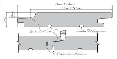
Allowances have been made for expansion gaps, but must be implemented using a 6mm spacer to achieve a uniformed shadow line.
