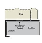
\* 9mm x 1.6mm gaskets are factory fitted. Additional foam gaskets, to form second moisture barrier, are available in rolls for on-site installation, or alternative sealant method can be implemented.
